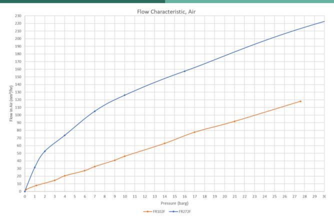
Flow characteristics above assume a pressure drop of 0.14 bar g across filter
